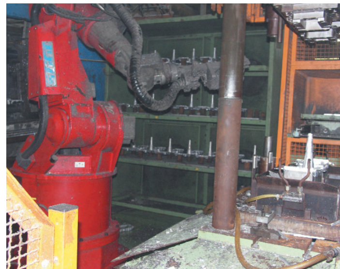
Removal robot with Triflex® R in the casting cell.
