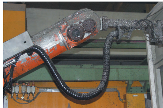
Moves in more than one dimension: Triflex® R, size 40.
